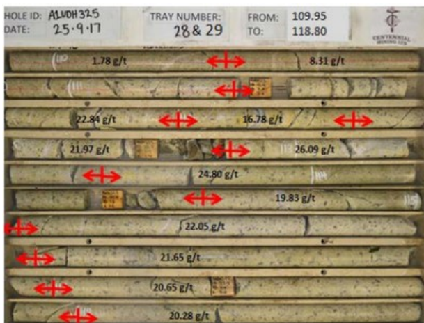
Figure 4-4: High Grade Diamond Drill Core from Altered Dyke Style Mineralisation
